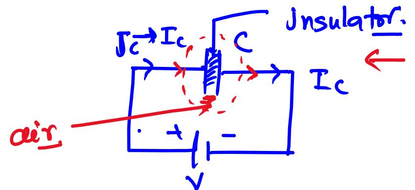
There is some way in which current flows through the free space or insulator between the parallel plates of the capacitor.
