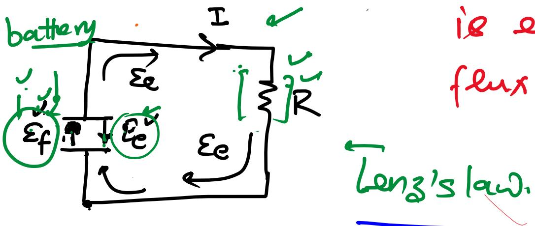
The induced emf,  $V_{emf}$  (v) in any closed path is equal to the time rate of change of flux linkage.
