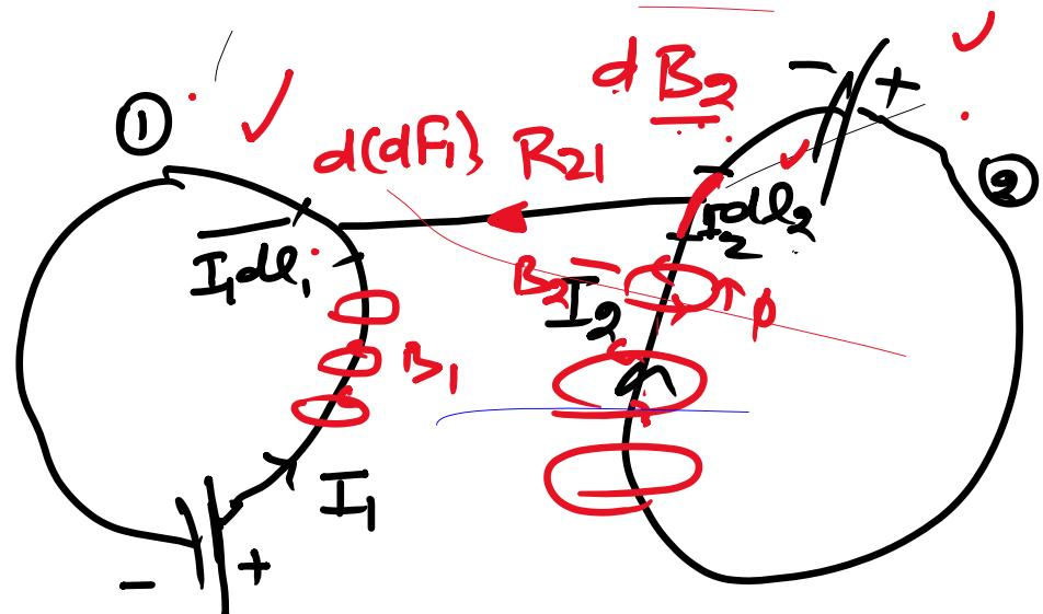
$$\underline{dB}_2 = \frac{\mu_0 I_2 d\underline{l}_2 \times \hat{aR}_2}{4\pi R_{21}^3}$$
