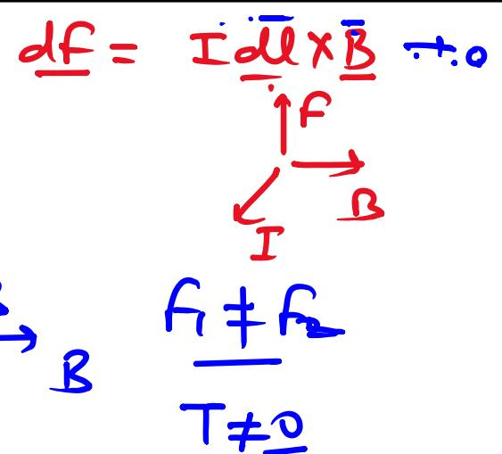
$$T = \omega \times F_0 = \omega F \sin \alpha \quad F_0 = \vec{B} \vec{l} I$$
