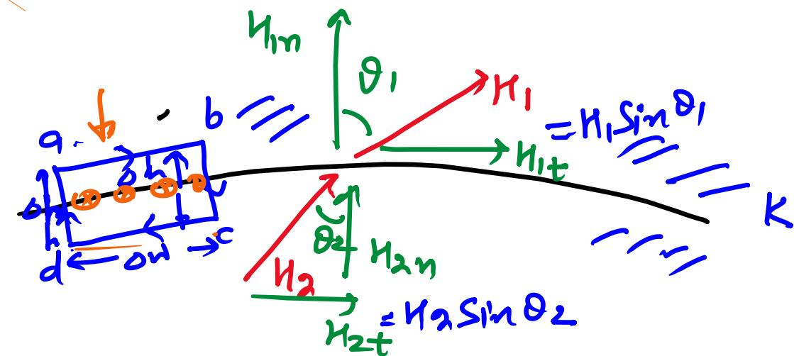
$$\oint \mathbf{H} \cdot d\mathbf{l} = I = K \omega \Rightarrow K \omega = H_{1t} \Delta W + H_{1n} \frac{\partial h}{2} + H_{2n} \frac{\partial h}{2} - H_{2t} \Delta W - H_{1n} \frac{\partial h}{2} - H_{2n} \frac{\partial h}{2}$$
